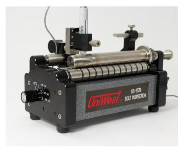
The strength of UniWest's tie-bolt inspection system is in the simplicity of the design. Using both gravity and thread angle, the probe is driven along the thread pattern and then manually manipulated along the rest of the shank and head radius. The entire inspection can be completed in less than seven seconds. There are no expensive fixtures to replace. All standard size tie bolts can be inspected with this one instrument. Special modifications can be made to fit over and undersized bolts.
