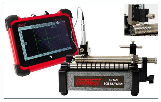
The strength of UniWest's tie-bolt inspection system is in the simplicity of the design. Using both gravity and thread angle, the probe is driven along the thread pattern and then manually manipulated along the rest of the shank and head radius. The entire inspection can be completed in less than seven seconds. There are no expensive fixtures to replace. All standard size tie bolts can be inspected with this one instrument. Special modifications can be made to fit over and undersized bolts.
